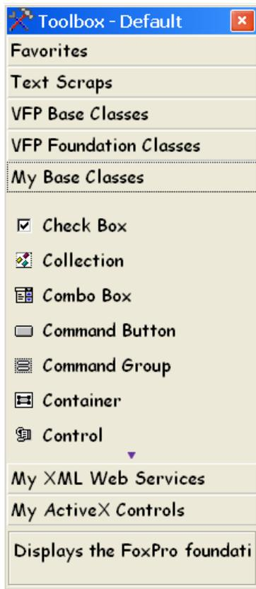
Figure 1. The Toolbox contains categories (the horizontal "buttons") and items. This figure shows the built-in categories. You can add your own, as well.
