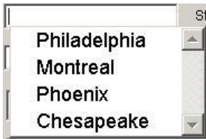
Figure 1. Using AutoComplete—This textbox for entering a city has AutoComplete set to show the list in most recently used order.
