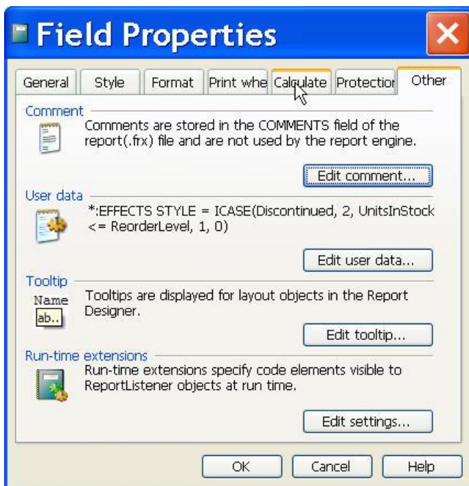
Figure 3. Specifying effects—Using the EffectsListener class, you specify formatting changes as User data.
