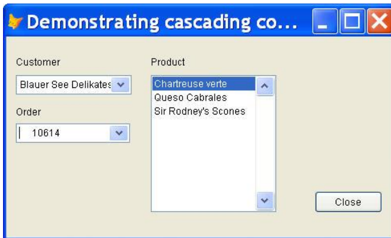
Figure 1. Cascading combos and lists—It only takes a little code to set up combos and lists to update when a selection is made in another list or combo.
