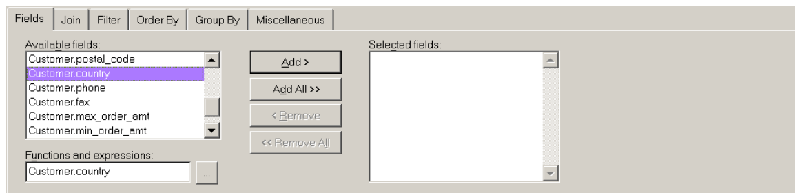
Figure 8. Ease of use—When you click on a field in the Available fields list, it's copied into the Functions and expressions textbox, where you can edit it or quickly move to the Expression Builder.
