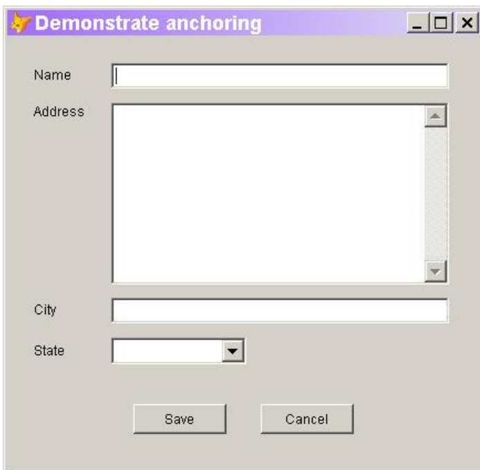
Figure 1. Prepared for resizing—The Anchor property for each control on this form has been set to keep it attractive as the form size changes.
