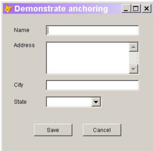
Figure 1. Prepared for resizing—The Anchor property for each control on this form has been set to keep it attractive as the form size changes.
